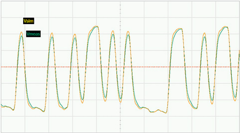
Figure 10. Waveforms V_{meas} and V_{sim} of probe loading example
