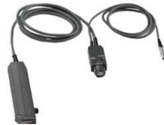
The N2783B current sensor has 100 MHz bandwidth, and 100mV/A sensitivity
