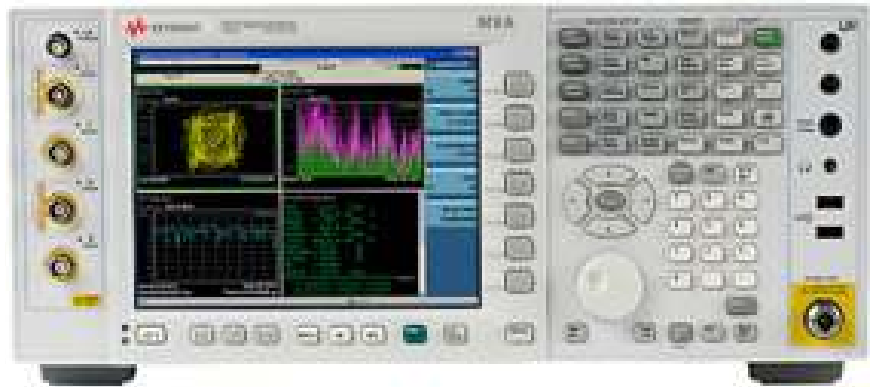
16 bit resolution baseband and high performance RF inputs make the N9030A PXA signal analyzer an ideal tool for all RF PA evaluation tests.
