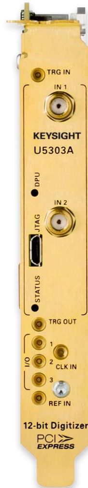
Figure 3. U5303A front panel with analog inputs and multiple I/O signals.
