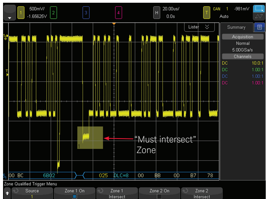
Figure 11: Using InfiniiScan Zone Trigger to synchronize on just frames that include arbitration.
