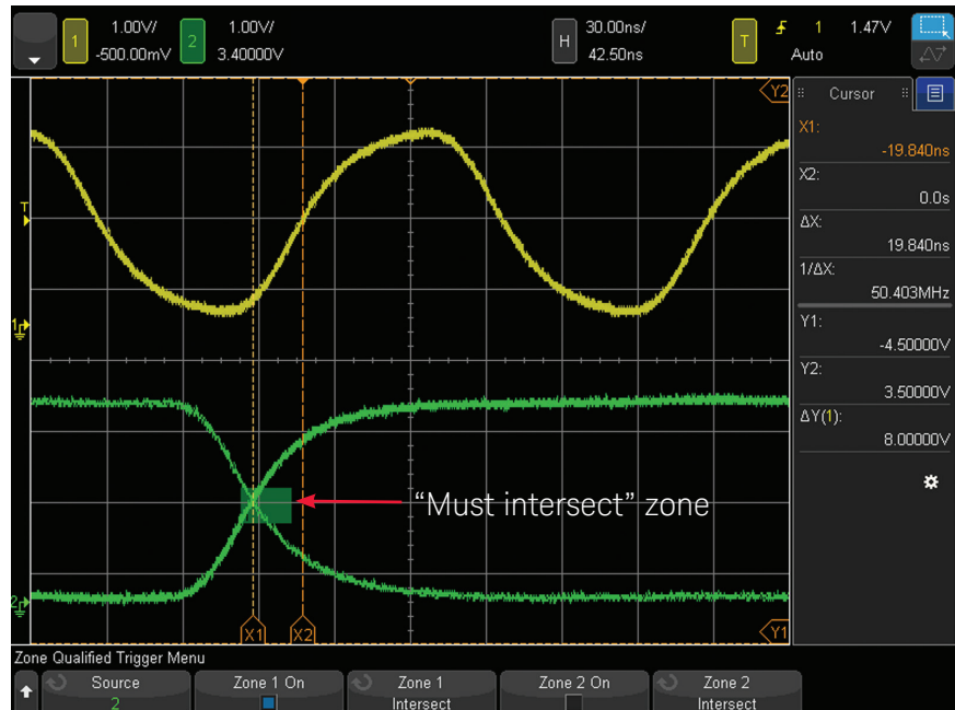
Figure 5: Using InfiniiScan Zone Trigger to isolate setup time violations.
