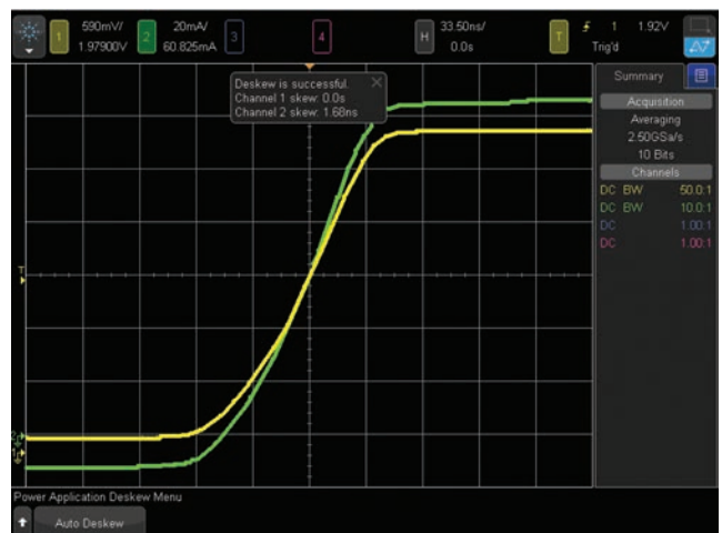
Figure 7: Deskew display after completing automatic deskew between voltage and current probes.
