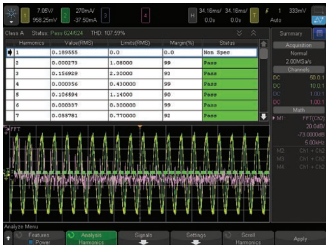
Figure 11: Current Harmonics measurement in a tabular format.
