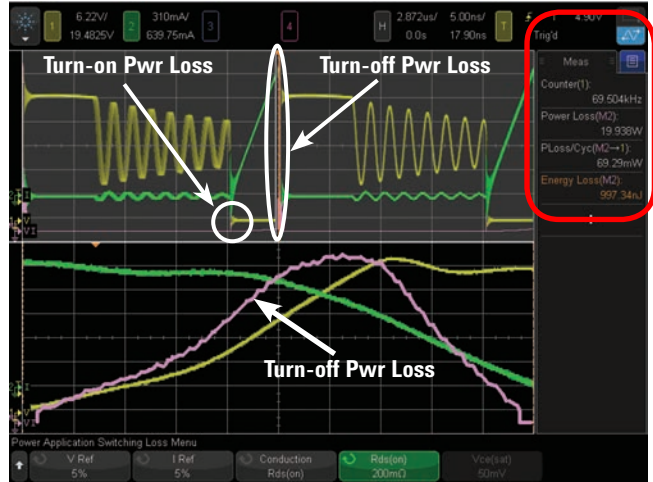
Figure 18: Windowing-in on the power spike at center-screen to measure the power and energy loss during just the transistor's turn-off phase.
