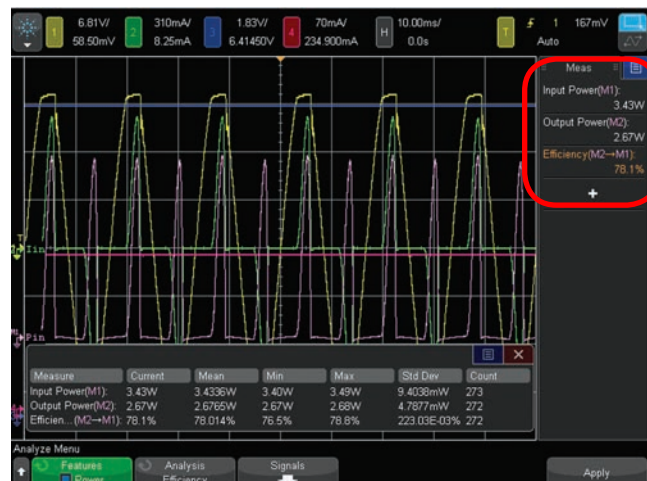
Figure 39: Power Efficiency measurement results. .
