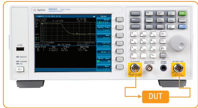
Figure 8. Option TG7 (tracking generator) provides scalar network analysis capability up to 7 GHz
