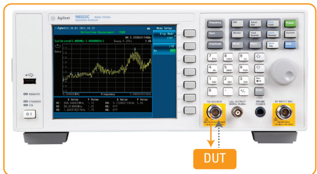
Figure 9. Option RM7 provides reflection measurement capability up to 7 GHz
