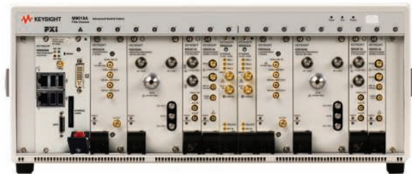
Two-channel Keysight M9392A PXI vector signal analysis system (50 MHz to 26.5 GHz) includes the M9036A controller, 2 of the each of the following: M9302A local oscillator modules, M9360A attenuator/preselector modules, M9361A downconverter modules, M9351A downconverter modules and M9202A IF digitizer modules placed within the M9018A PXI 18-slot chassis.
