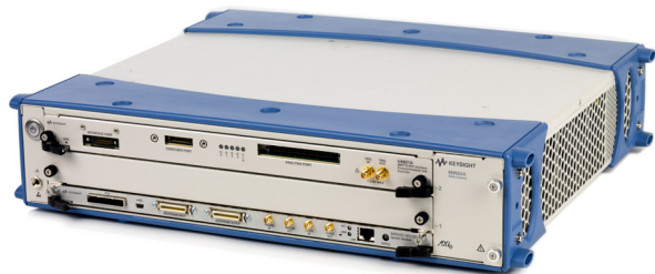
Combine multiple modules in a 2 (M9502A) or 5 (M9505A) slot AXIe mainframe to analyze and simulate cross-system behavior.
