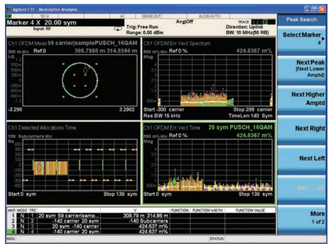
Figure 4. Uplink modulation analysis measurement showing constellation, EVM vs. subcarrier, detected allocation, and EVM vs. symbol information. Measurements are color-coded based on channel type and up to 12 markers with marker coupling between measurements are used for ease of troubleshooting.
