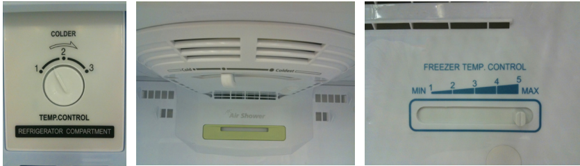
Figure 1. Temperature controllers found on refrigerators
