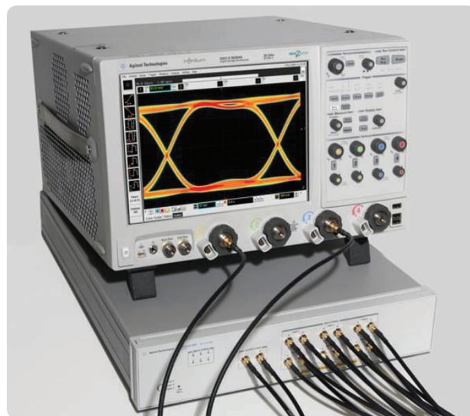
Figure 14. Automated testing for multi-lane digital bus interface through switching solution switch matrix.
