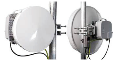
Figure 2. P2P transceiver modules (photography provided courtesy of Sub10)
