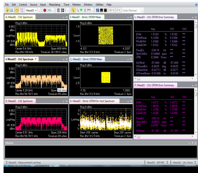
Figure 3. The N9070A is downconverting two 802.11ac signals (160 MHz bandwidth each) that are adjacent to each other. The 89600 VSA has multi-measurement capability to analyze both signals simultaneously. Note span of 400 MHz.
