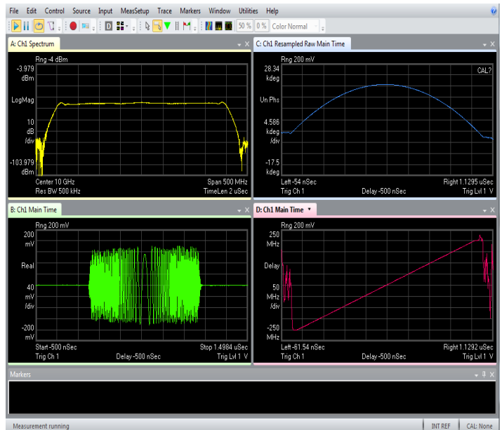
Figure 2. Analysis of a wideband chirp and evaluation phase and frequency across the band.
