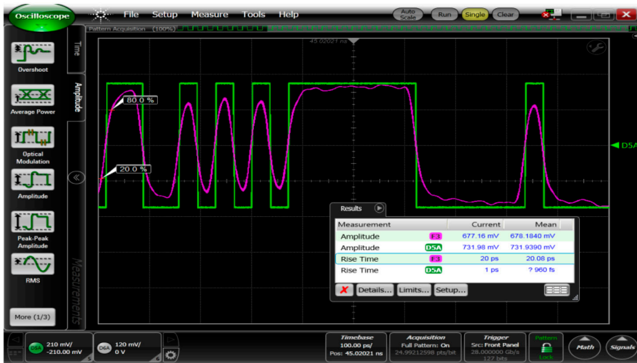
Figure 17: Predicted waveform at the output of the fixture (F3 Pink) when using an ideal 28G input signal (D5A Green).
