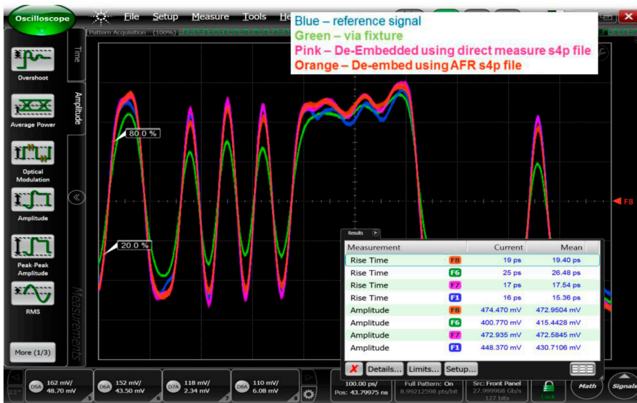
Figure 29: Waveform comparison showing good correlation between de-embedded signal using direct probe measurement model (F7 pink) and AFR model from the calibration 2x test fixture trace (F8 orange).
