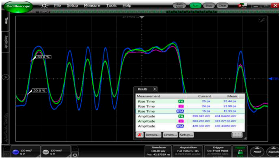
Figure 25: The simulated signal (F2 Pink) and actual signal (F6 Green) show good correlation, especially on 1010 bit and isolate bit sequences (most important).
