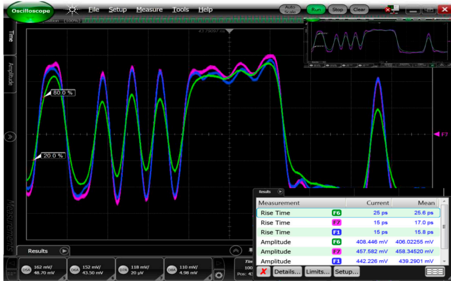
Figure 27: De-embedded signal (F7 pink) compared to reference trace (F1 blue) shows good correlation and provides further model validation.
