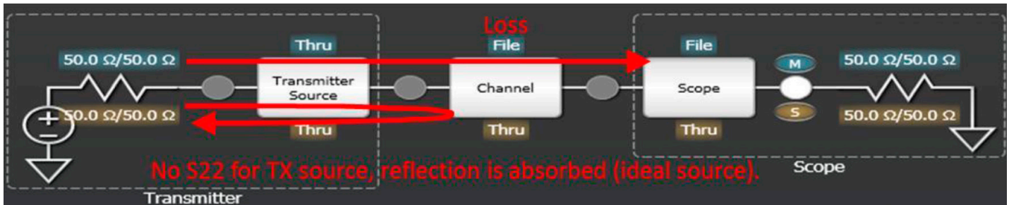
Figure 12: Partial de-embedding: The DUT (left) is assumed to be ideal, so any reflections from the fixture are assumed to be absorbed and are ignored when partial de-embedding is implemented.
