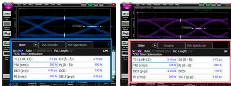
Figure 28: Jitter measurement comparison of de-embedded signal and reference signal; good ISI correlation (measured and de-embedded ISI is 4.88ps) which further validates the model.
