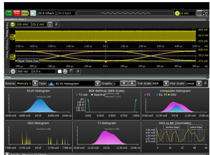
Figure 12. Real-world jitter measurements using Infiniium S-Series oscilloscopes. All models in the family utilize the same time base technology block and a low horizontal component of jitter measuring less than 130 fs over short record lengths.
