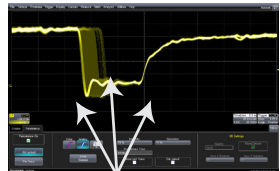
6Zi after 60 seconds using "WaveStream" Fast Viewing Mode – it never sees the glitches and shows limited signal jitter due to its slow update rate.
