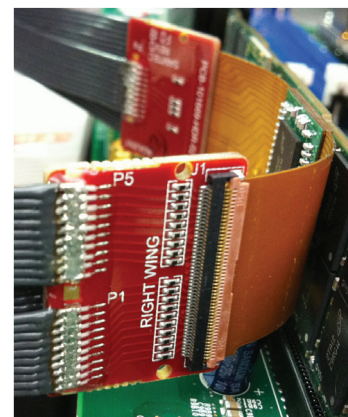
Figure 1. E5849A 46-ch single-ended ZIF probe for x4/x8 DRAM BGA interposer connects to 90-pin logic analyzer cables
