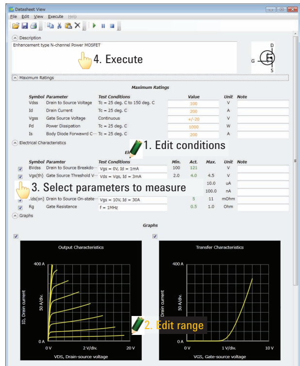
The intuitive data sheet characterization mode provides complete device characteristics in a few simple steps
