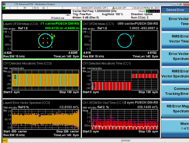
Figure 3. Uplink modulation analysis measurement showing constellation, EVM vs. subcarrier, detected allocation, and EVM vs. symbol information for two component carriers. Measurements are color-coded based on channel type and up to 12 markers with marker coupling between measurements are available for easier troubleshooting.
