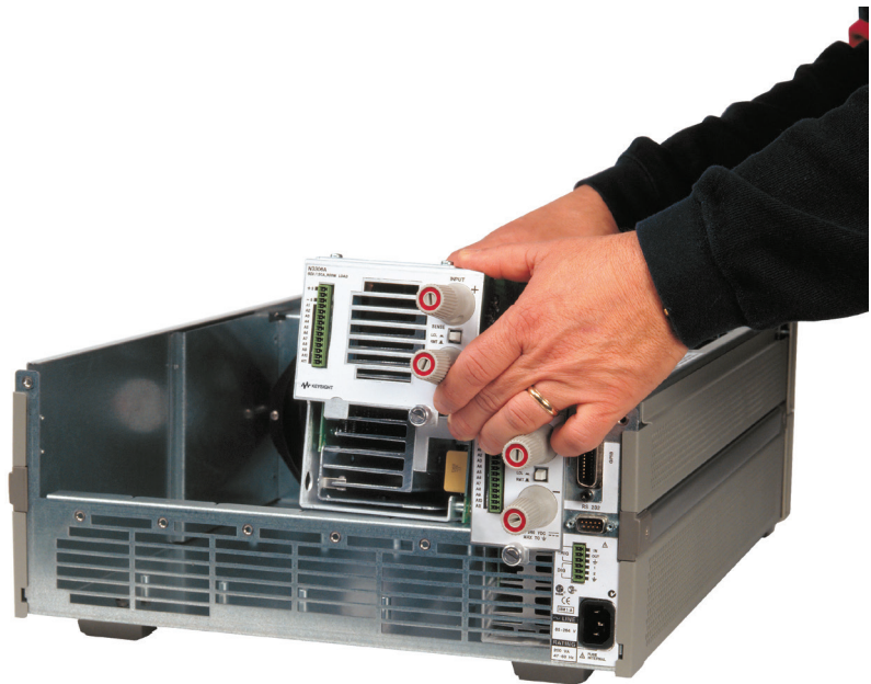
N3300 Series Loads can be configured with load modules ranging from 150 – 600 W
