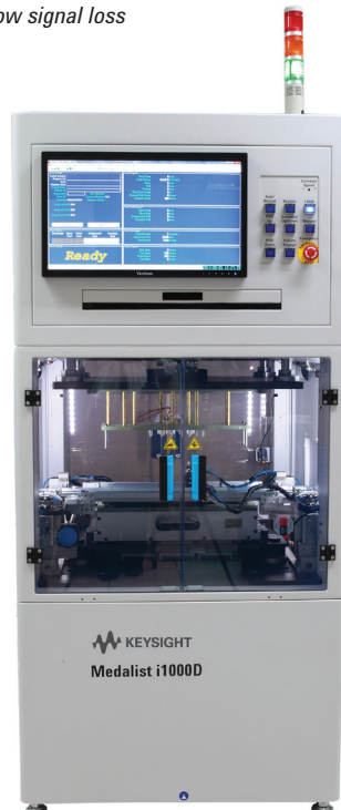
i1000D Small Footprint Inline In-Circuit Test System
