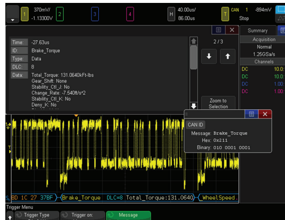
CAN-dbc symbolic trigger and decode
