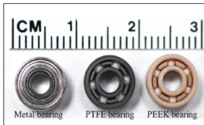
Figure 2. Optical images of bearing samples top view [1].
