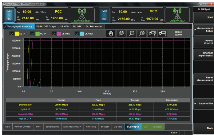
The UXM provides stable, bidirectional end-to-end data throughput
