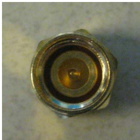
Figure 2. The male short circuit cap, top view and side view
