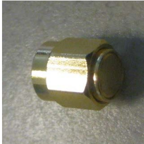
Figure 2. The male short circuit cap, top view and side view
