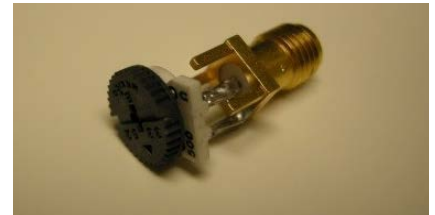
Figure 6. The variable 500 Ω potentiometer load
