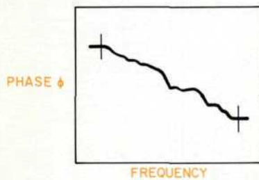
Figure 10. Phase Response versus Frequency for Device with Large Electrical Length.
