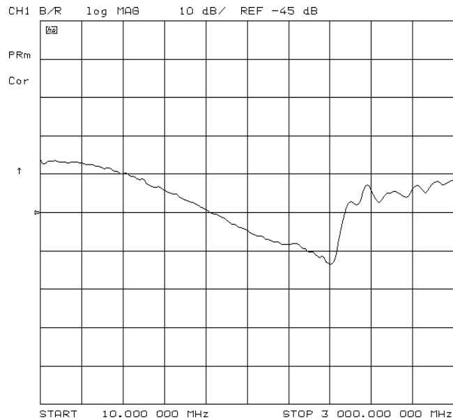
Figure 2-35 Example Mixer LO to RF Isolation Measurement
