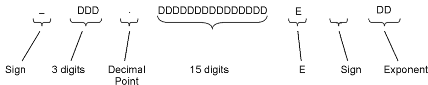
Figure 4-1 FORM4 (ASCII) Data-Transfer Character String
