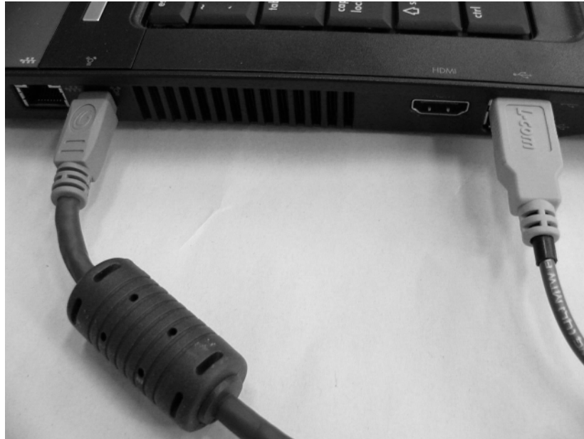
Figure 1-18 IEEE-1394 cable connected to laptop PC (left side of image). EMC grounding cable connected to laptop PC (right side of image).
