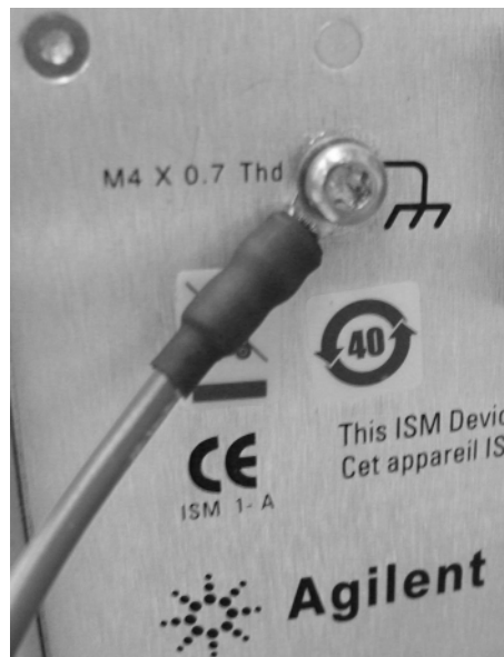
Figure 1-17 EMC grounding cable attached to VXI main frame chassis
