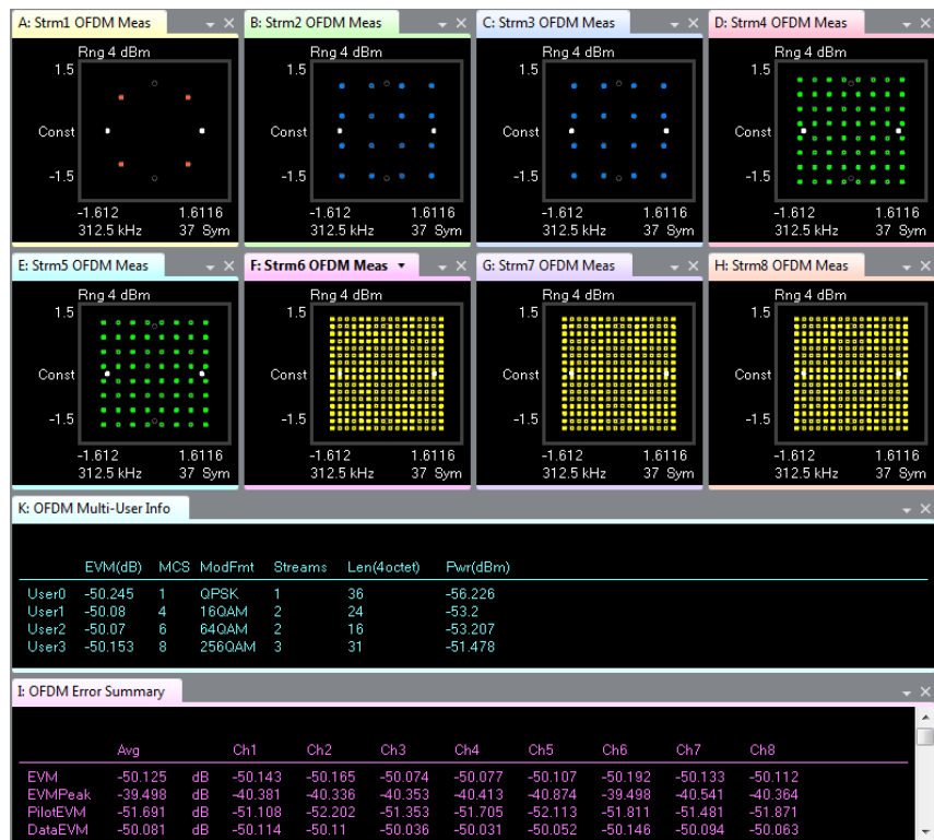
View key 802.11ac MIMO parameters such as multiple constellations, error summary and multi-user info for up to 8 transmit streams simultaneously.
