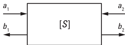
Figure 2. S-parameters for 2-port network
