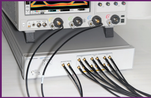
SMA connection test interface
