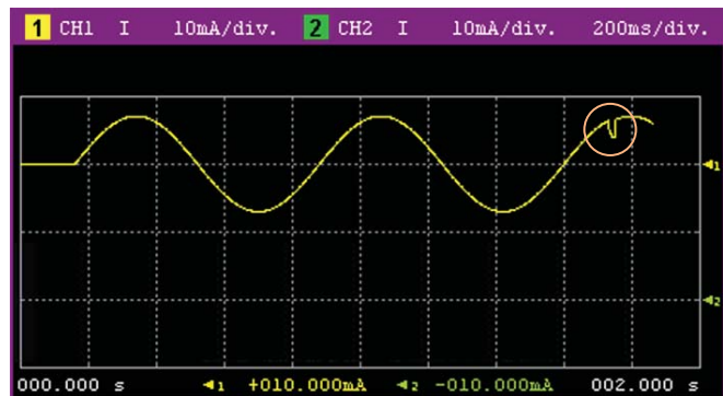
Roll view mode allows you to capture low-frequency transient phenomena.
