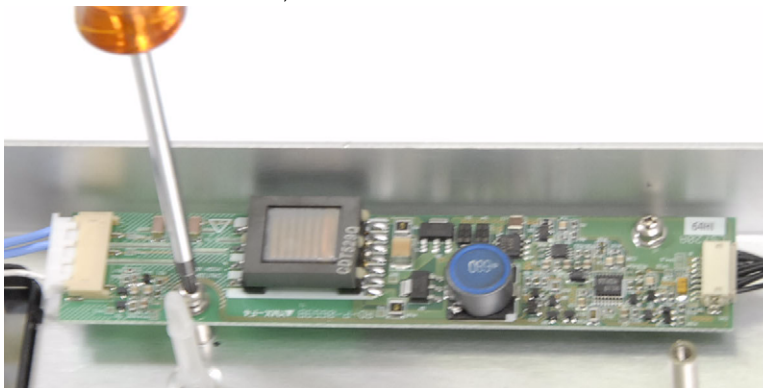
Figure 24 Removal of inverter board
