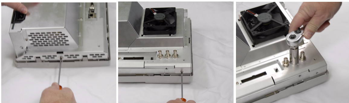
Figure 19 Removing the rear deck assembly
