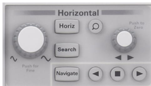
Figure 4 Oscilloscope horizontal (X-axis) controls
