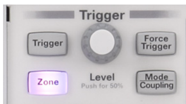
Figure 6 Oscilloscope trigger level control
