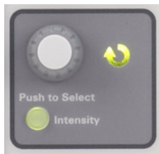
Figure 7 Oscilloscope general-entry control
