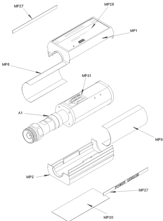
**Figure 10 Illustrated Parts Break down**
