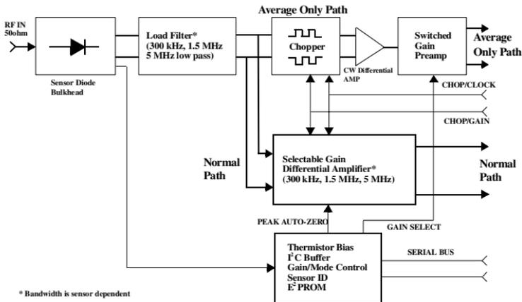
**Figure 11 Simplified Sensor Block Diagram**
