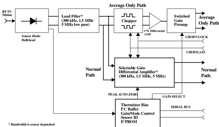
**Figure 1 Simplified Sensor Block Diagram**
