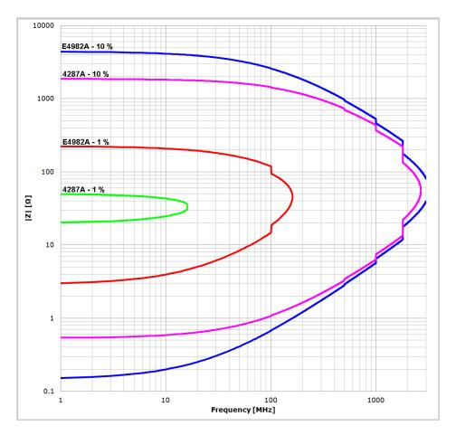
The setting for the above: Oscillator Level: 1 dBm (for E4982A) & 0 dBm at > 1 GHz (for 4287A), Averaging Factor < 8, Measurement Speed of E4982A: Mode 3, Temperature Deviation  $\leq$  5 °C
