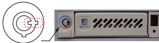
Figure 2-5 Removable Hard Disk Drive
