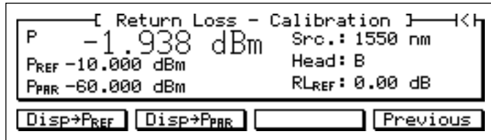
Figure 3-5 Return Loss Calibration Display
