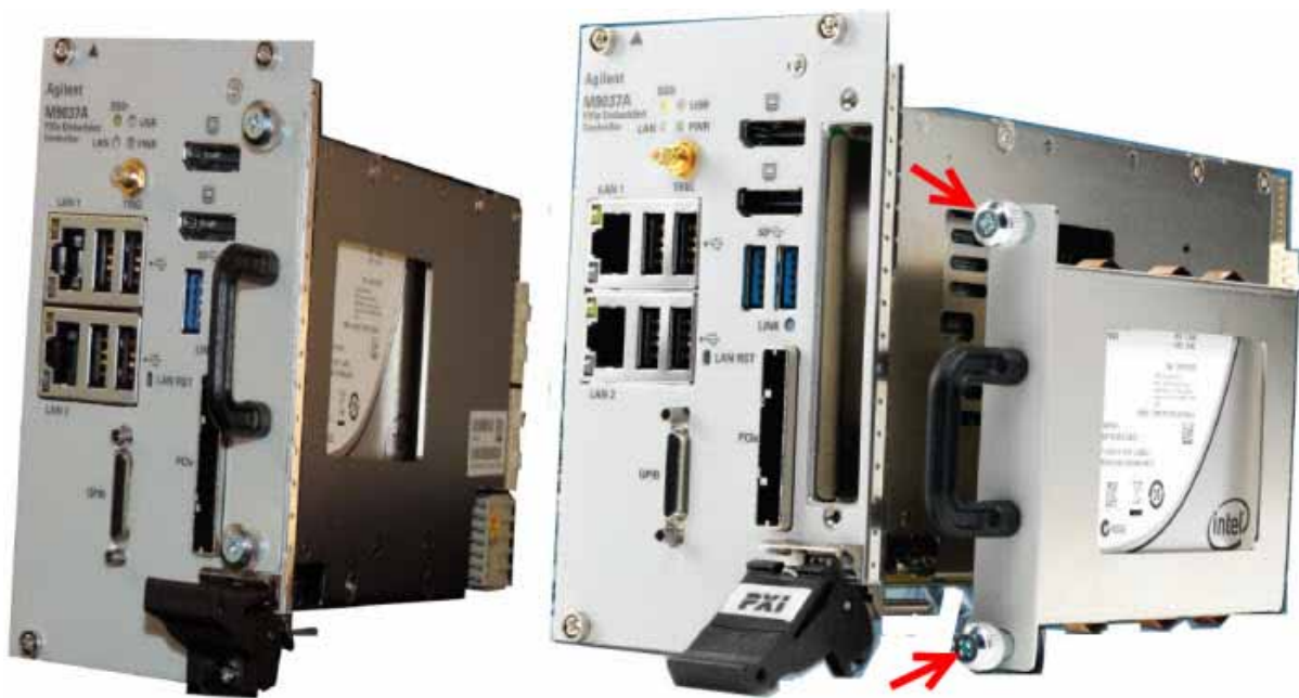
Figure 5-2 Removing the solid state drive (Keysight M9037A controller)
