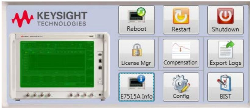
The E7515A Control Panel enables you to interact with and manage the hardware components of the UXM. It is always running if the test set is turned on. If it is not displayed on the screen, it is minimized in either the lower left or right area of the Windows task bar.
