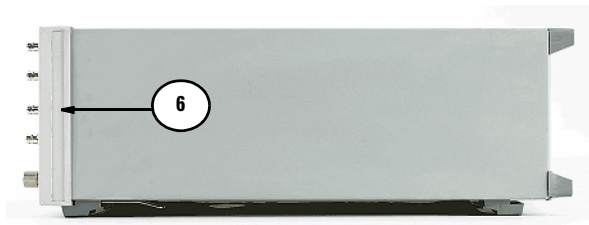
Figure 2-36 Trim-Side Overlay (Installed)
