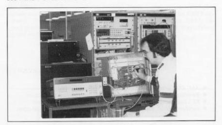
The 8901A is an excellent trouble-shooting tool when used with a high impedance probe such as the HP 1120A 500 MHz active probe. It can monitor signals at various points of a device. At each point, the residual noise, AM content, FM content, distortion and signal level can be checked. In this way, any element that creates AM to FM conversion, additional noise, or additional distortion can be isolated.
