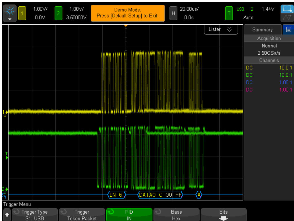
Figure 91 Triggering on IN Token packets.
