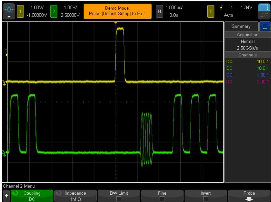
Figure 44 Capturing a complex burst signal while triggering on a synchronization signal.
