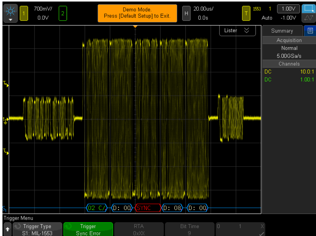
Figure 100 Triggering on a unique sync error.
