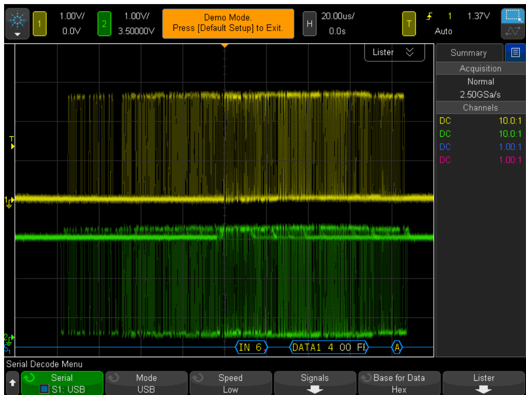
Figure 90 Fast, hardware decoding of USB traffic.
