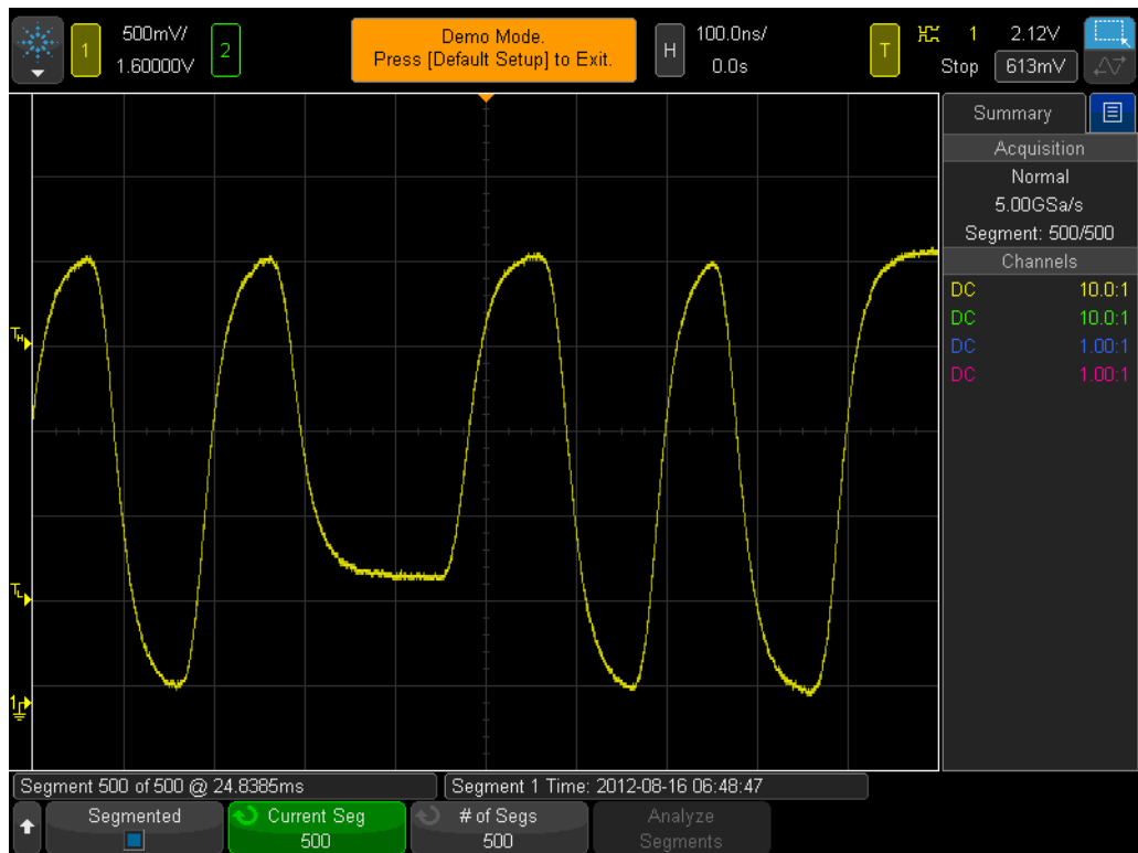
Figure 40 Using the scope’s Segmented Memory acquisition to selectively capture 500 consecutive runt pulses.
