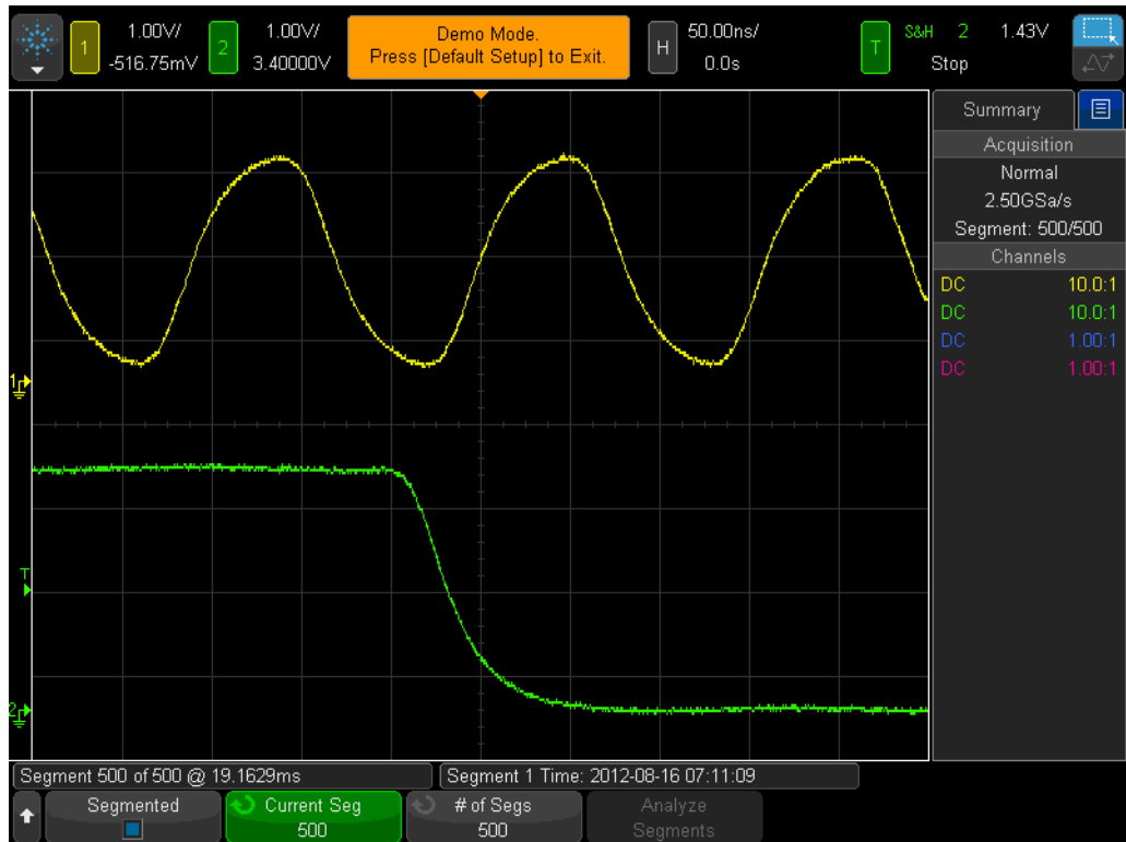
Figure 43 Using the scope's Segmented Memory acquisition to selectively capture 500 consecutive occurrences of a setup time violation runt pulses.
