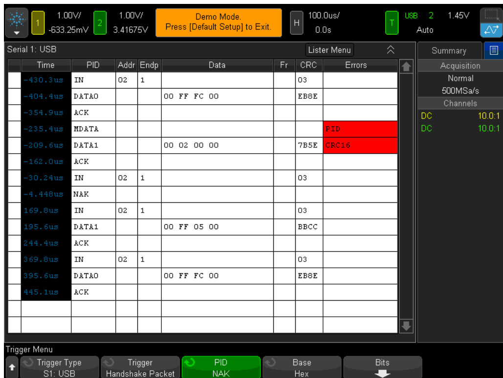
Figure 92 Using the full screen lister to view decoded information.
