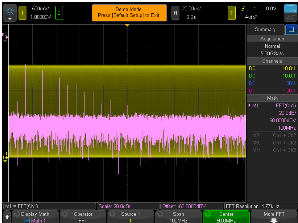
Figure 12 Performing an FFT math function on a repetitive digital clock.
