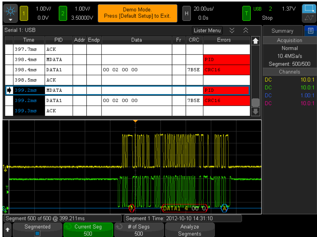
Figure 93 Using the scope's Segmented Memory acquisition to selectively capture more USB traffic.
