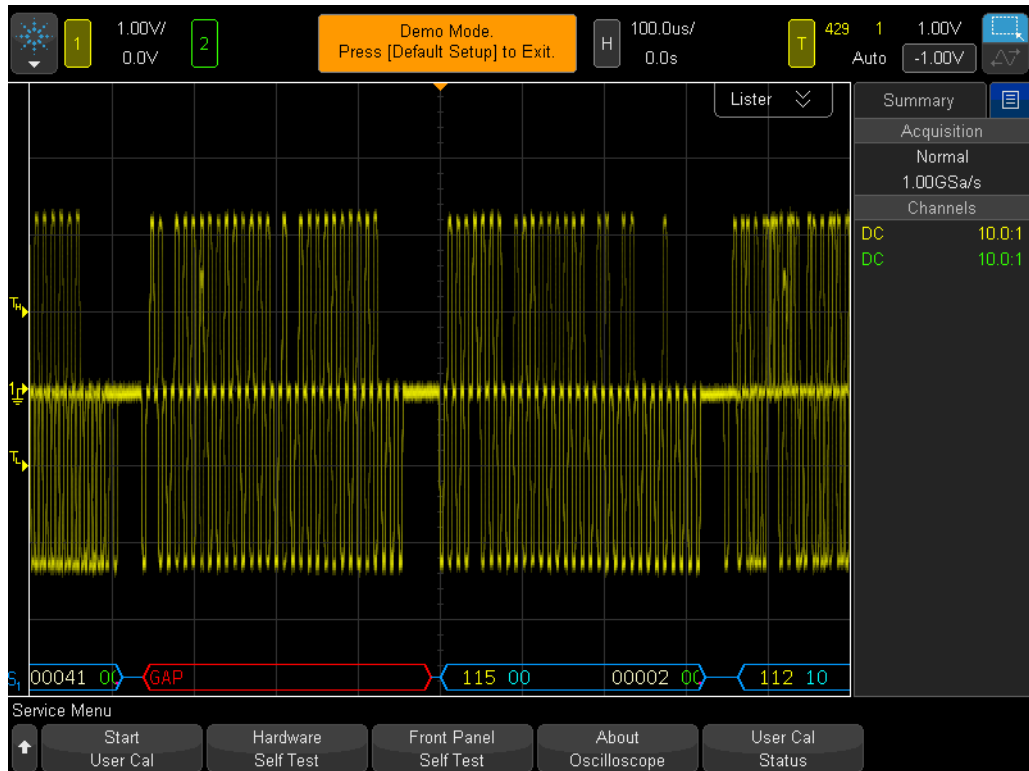
Figure 95 Fast hardware decoding of ARINC-429 traffic.
