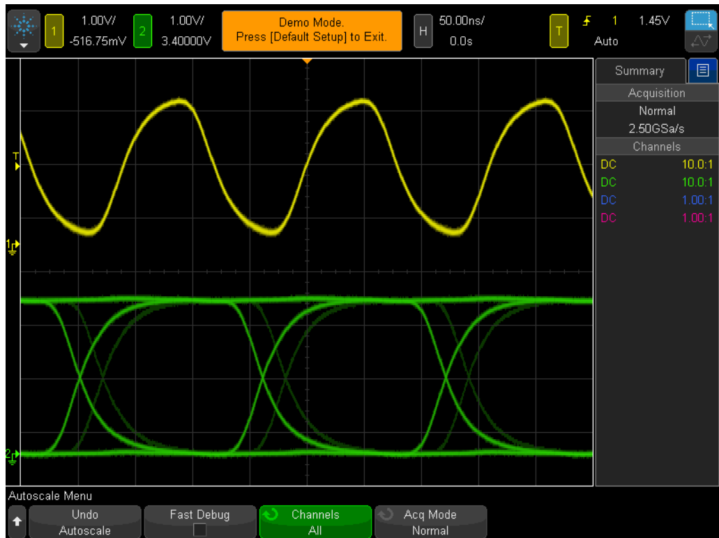
Figure 41 Display of a clock signal (yellow trace) and data signal (green trace) in the form of an eye-diagram.
