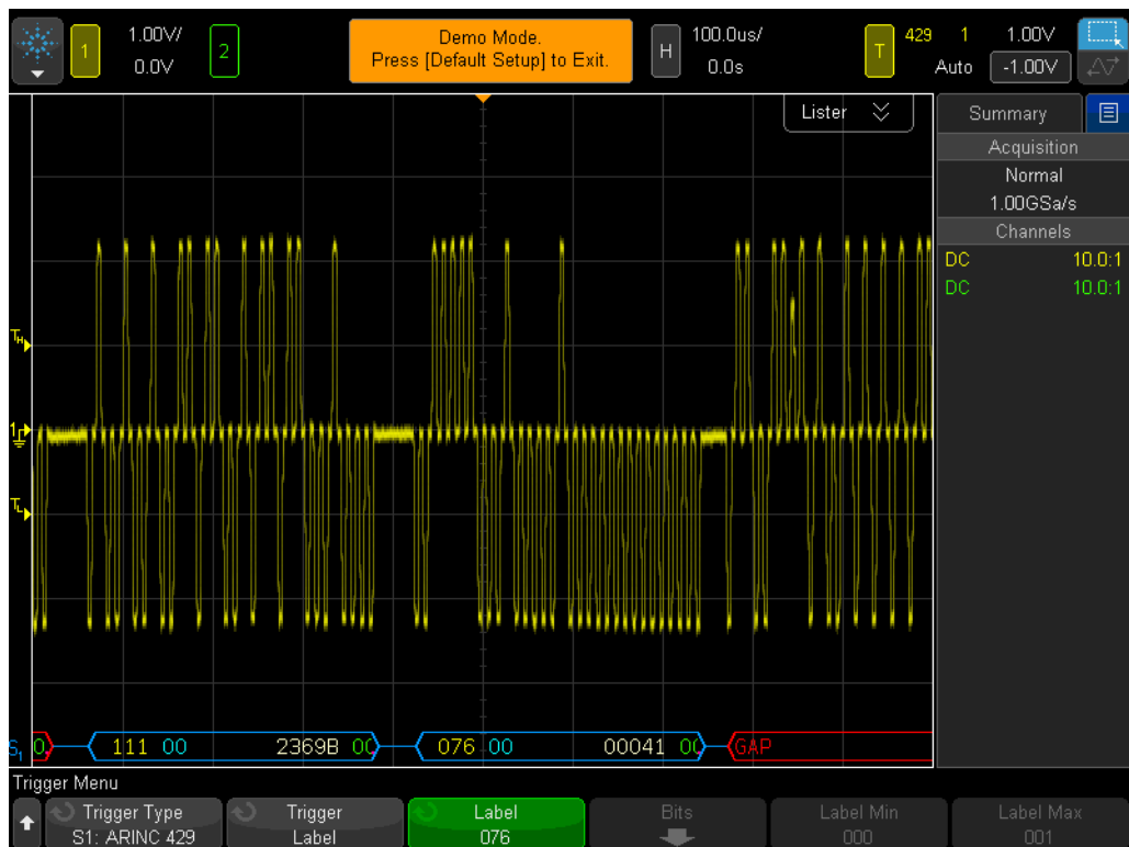
Figure 96 Triggering on a frame with label 076.
