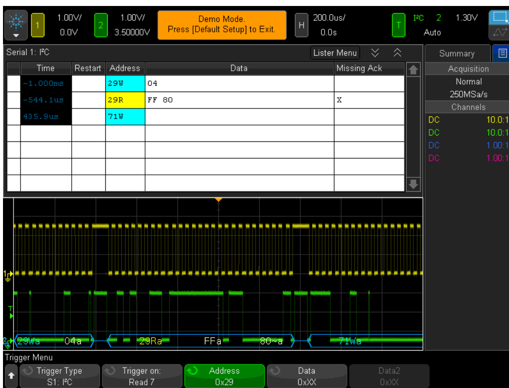
Figure 52 Triggering on I 2 C traffic.
