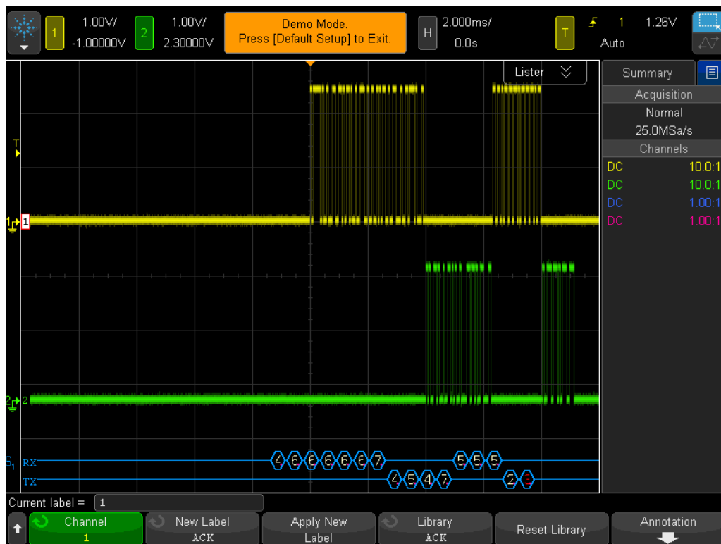
Figure 61 Decoding the RS232/UART serial bus.
