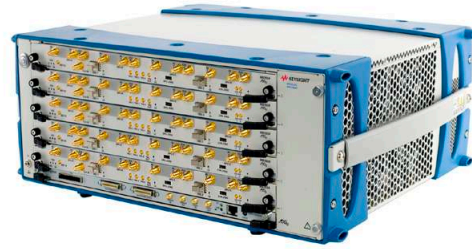
Figure 1. M9703A AXIe 12-bit digitizer and M9536A embedded AXIe controller in M9505A 5-slot chassis.
