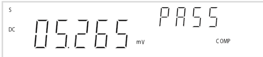
Figure 2-5 Typical Comp operation display
