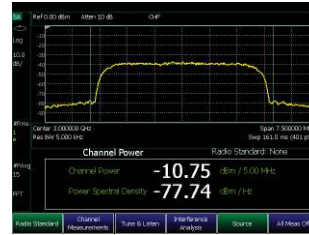
Channel power measurement
