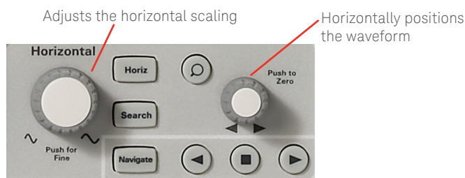
Figure 17. Front panel horizontal control section on a Keysight InfiniiVision 2000 X-Series oscilloscope
