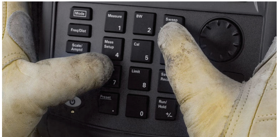
Figure 3. A portrait orientation coupled with sufficiently large front-panel buttons enables easy operation, even when wearing gloves.
