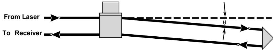
If the Agilent 10702A Linear Interferometer is placed in a beam which has been aligned parallel to the motion of travel, the outgoing beam can be deflected by as much as 30 arc-minutes ( $\theta$ ) due to the incoming-outgoing beam parallelism specifications of the Agilent 10702A interferometer. This could cause not only cosine error but also possible loss of signal during movement of the Agilent 10703A Retroreflector.
