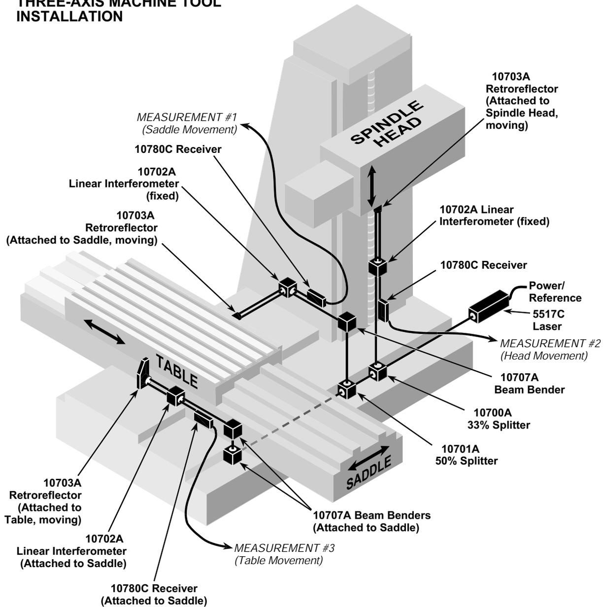
**Figure 7A-3. Three-axis machine tool Installation**
