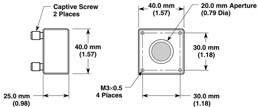
Figure 7A-13. Agilent 10767A Linear Retroreflector — dimensions
