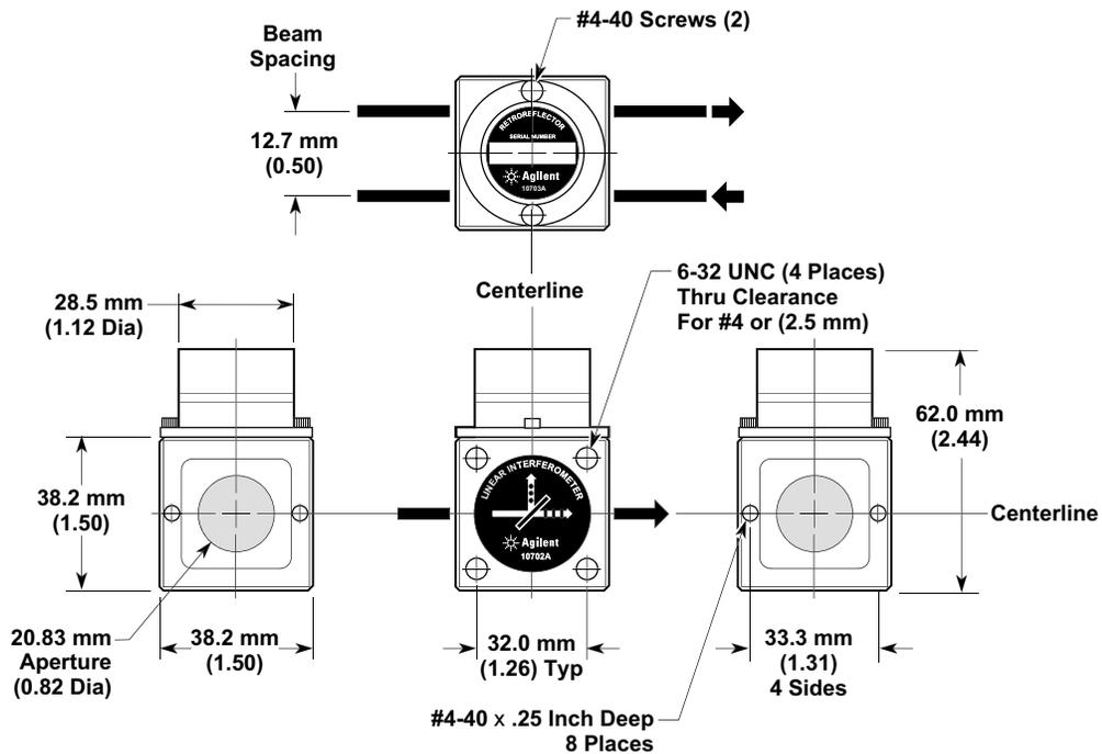
Figure 7A-8. Agilent 10702A Linear Interferometer — dimensions
