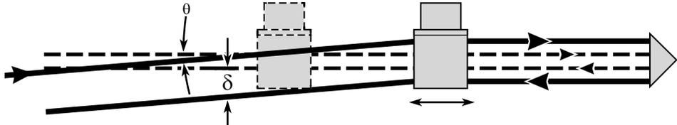
If the Agilent 10702A Linear Interferometer, instead of the Agilent 10703A Retroreflector, is moved during the measurement, the beam in the measurement path will remain parallel, but will be displaced. This displacement  $\delta$  will occur at the receiver, causing a decrease and eventual loss of signal, depending on the distance traveled.
