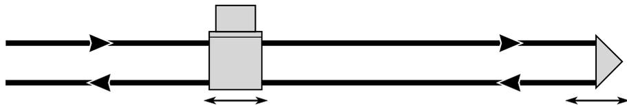
If motion of the linear interferometer is required, the Agilent 10702A-001 Linear Interferometer with Windows should be used. This provides special wedge windows which makes the outgoing beam parallel to the incoming beam. This allows motion by either the Agilent 10703A Retroreflector or the Agilent 10702A-001 Linear Interferometer.
