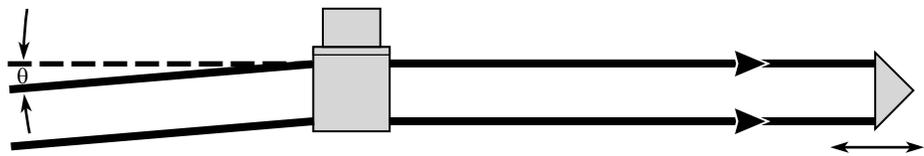
To compensate for this, alignment is performed with the Agilent 10702A Linear Interferometer in place. This allows the laser beam to be aligned parallel to the motion of travel to minimize cosine error and maximize signal. Since the incoming beam is now not parallel to the motion of travel, the Agilent 10702A Linear Interferometer must remain stationary. (See below).
