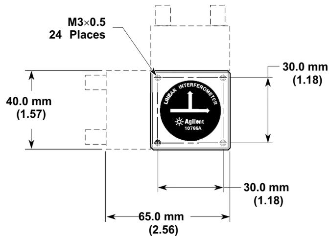
Figure 7A-12. Agilent 10766A Linear Interferometer — dimensions
