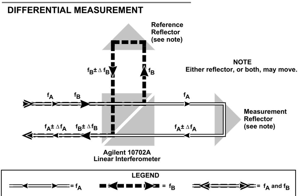
**Figure 7A-7. Differential measurements with the Agilent 10702A**
