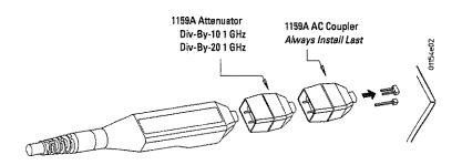
The 1159A probe's best performance is achieved when the probe attenuation is set to /10 in the Infinitum's Probes Setup dialog box.
