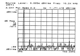
The default frequency span is 0 Hz to 102.4 kHz. The 10.24 kHz test signal thus appears at the left side of the analyzer's display, near the first graticule line from the left.
