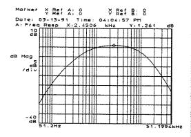
This moves the marker to the largest part of the frequency response trace. Because we are looking at a frequency response trace, the Y-marker indicates the gain (or loss) of the network-under-test.
