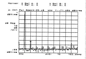
This brings up the marker menu and then moves the marker to the largest frequency component on the display—in this case, the 10.24 kHz fundamental.
