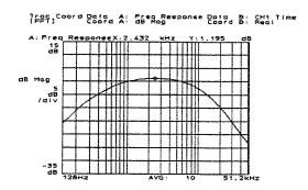
This moves the marker to the largest part of the frequency response trace. Because we are looking at a frequency response trace, the Y-marker indicates the gain (or loss) of the network-under-test.
