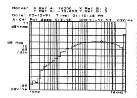
This turns on the analyzer's channel 1 input A-weight filter. An A-weight filter is useful for acoustics measurements and for characterization of audio-frequency devices since its response simulates that of the human ear.
