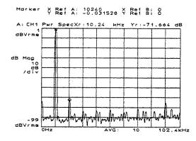
Note how the Y-axis marker readout indicates a relative reading of approximately -72 dB, and the X-axis marker shows the frequency offset from the fundamental (around 10 kHz in this case).
