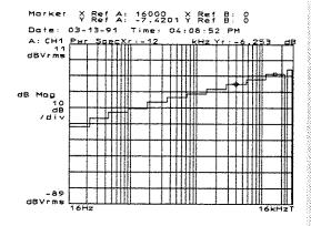
Random noise—often called white noise or gaussian noise—has its energy distributed equally across all frequencies (constant bandwidth). In contrast, pink noise has its energy distributed equally per octave (proportional bandwidth). In a moment, we'll demonstrate the difference between these two noise sources.
